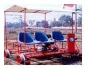
**INTRODUCTION:** - Light Weight Motorized Trolley is an efficient machine in the hands of permanent way inspector which facilitates him with an easy riding method while inspecting the running tracks. The trolley nullifies the need of two trolley men as it is fitted with a strong engine for pushing operation.
